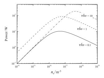
Figure 7.6 Absorbed power as a function of the electron density for fixed coil current and for three values of the ratio  $v_m/\omega$ ;  $I_{coil} = 3 \text{ A}$ ,  $r_0 = 0.065 \text{ m}$  and l = 0.3 m.
