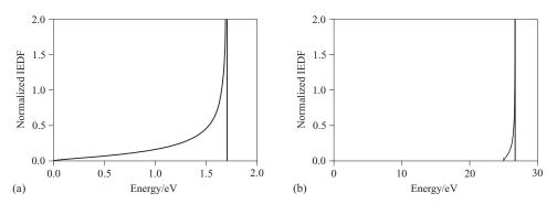
Figure 4.5 The ion energy distribution function from a Tonks–Langmuir model with  $kT_e/e = 2$  V (a) at the plasma/sheath boundary – the maximum ion energy corresponds with ions falling through  $0.854kT_e/e$  and (b) after collisionless acceleration through a 25 V DC sheath – the entire distribution is shifted up the energy axis by the potential across the sheath.
