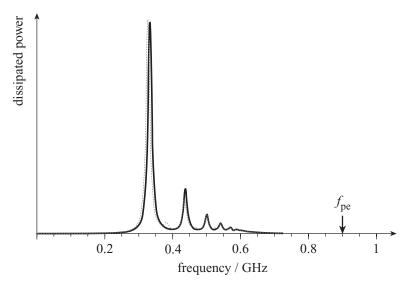
Figure 10.24 Calculated absorption spectrum of a multipole resonator.
