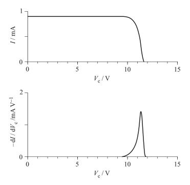
Figure 10.17 Current–voltage and the differential current–voltage characteristics for an RFA with an aperture of  $10^{-4}$  m<sup>2</sup>, when the ions enter the sheath with a distribution like that in Figure 4.5 and are then accelerated through a sheath potential of 9.6 V. This particular RFA has an energy resolution of 0.4 eV.
