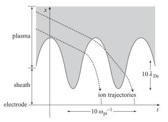
Figure 4.3 Schematic ion trajectories in a temporally modulated sheath ( $\omega \sim \omega_{pi}$ ): ions approach the sheath boundary close to the Bohm speed, being significantly accelerated when inside the sheath.
