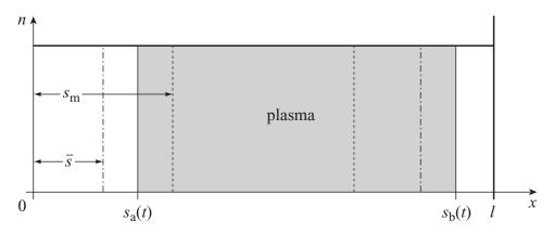
Figure 5.2 Schematic of the sheath dynamics for the constant ion density model.
