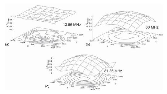
Figure 6.13 Maps of the ion flux to the electrode at 28 Pa/50 W for 13.56 MHz, 60 MHz and 81.36 MHz. The electrode separation was 4.5 cm, the electrode dimensions were  $40 \text{ cm} \times 40 \text{ cm}$ .
