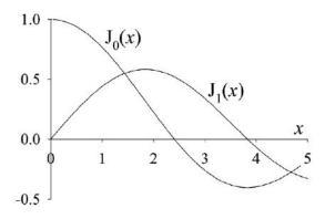
Figure 6.8 Zero-order and first-order Bessel functions.
