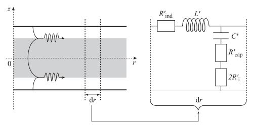
Figure 6.17 Schematic of the transmission line model constructed from the electromagnetic model.
