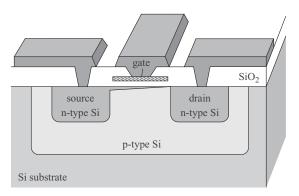
Figure 1.2 The structure of a silicon IC in the region of a MOSFET in which a gate electrode controls the formation of a channnel of n-type silicon between source and drain regions.
