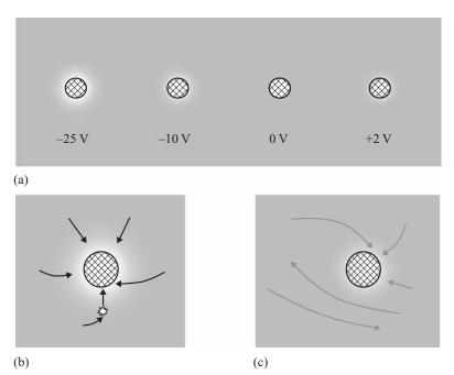
Figure 10.7 Schematics of a cylindrical (or spherical) probe. (a) Sheath development around a biased probe – the potential indicated is referenced to the plasma  $(\phi_p)$ ; (b) example ion trajectories  $(\phi < \phi_p)$ ; (c) example electron trajectories in electron saturation  $(\phi > \phi_p)$ . The lighter regions represent net space charge: positive if  $\phi_p < 0$  and negative if  $\phi > \phi_p$ .
