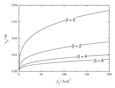
Figure 6.3 Sheath size as a function of the low-frequency current density amplitude  $J_0 = I_0/A$ , for the same conditions as in Figure 6.2.
