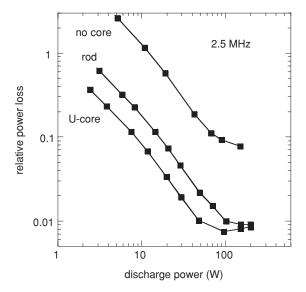
Figure 7.21 Relative inductor loss as a function of the discharge power with and without ferrite core. From [133].
