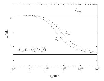
Figure 7.7 Total inductance  $L_{\text{ind}}$  and magnetic storage inductance  $L_{\text{m}}$  as a function of the electron density for  $v_{\text{m}}/\omega = 1$ . We have chosen N = 5,  $r_0 = 0.065 \text{ m}$ ,  $r_c = 0.08 \text{ m}$  and l = 0.3 m.
