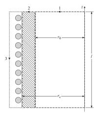
Figure 7.4 Ampère contours for the current in the plasma (1), in the dielectric tube (2) and in the coil (3).
