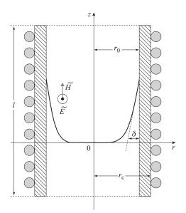
Figure 7.2 Schematic of the inductive discharge. The discharge is contained in a dielectric tube of inner radius  $r_0$ , outer radius  $r_c$  and length  $l \gg r_0$ . The induced electric field is azimuthal, while the induced magnetic field is axial. At high plasma density, both fields decay within the skin depth  $\delta$ .
