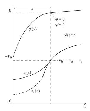
Figure 3.5 Densities and potential around the plasma/sheath transition region.
