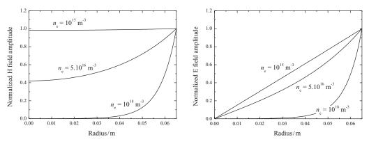
Figure 7.3 Calculation of the electromagnetic field magnitude normalized to the edge value at  $r = r_0$ , as a function of the cylinder radius and for various electron densities.
