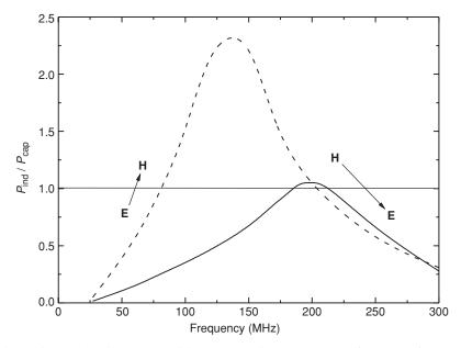
Figure 6.20 Inductive-to-capacitive power ratio,  $P_{ind}/P_{cap}$ , vs. frequency for  $n_{e0} = 5 \times 10^{17} \text{ m}^{-3}$ . The dashed line is for  $r_0 = 0.25 \text{ m}$  and the solid line is for  $r_0 = 0.15 \text{ m}$ . The other conditions are similar to those in Figure 6.18. From [21], where  $R_1$  is equivalent to  $r_1$  in this text.
