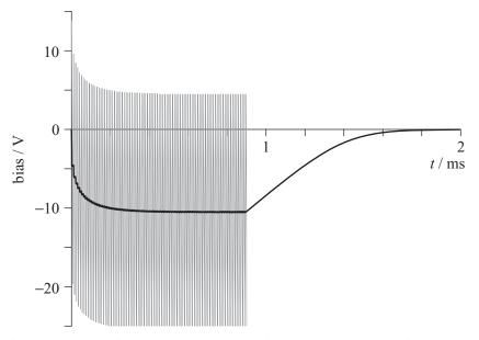
Figure 10.14 The instantaneous (unresolved, grey) and slow transient (black) potential of a self-biased planar probe of area  $1.8 \times 10^{-4}$  m<sup>2</sup> embedded in the grounded wall of a plasma source. Outside the chamber the probe is driven with a 0.9 ms burst of RF at 12 MHz and 15 V amplitude, applied through a 22 nF capacitor.
