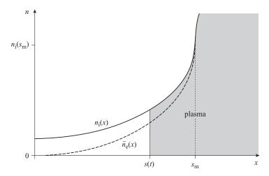
Figure 4.15 Charged particle densities in the vicinity of an RF Child–Langmuir sheath. The solid line shows the profile of steady ion density; instantaneous electron density is represented by the grey area and is delimited by x = s(t). The mean electron density is shown by the broken line. Ions enter the ion sheath ( $x = s_m$ ) at the Bohm speed and fall freely in the mean potential.
