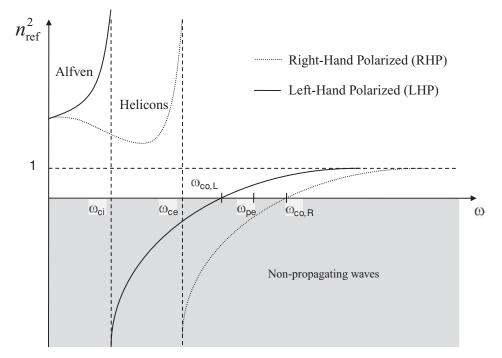
Figure 8.2 Square of the refractive index as a function of frequency for the LHP and RHP waves propagating parallel to the direction of  $B_0$  in an infinite magnetized plasma;  $\omega_{ce} \ll \omega_{pe}$ .
