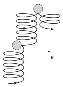
Figure 9.2 Schematic of electron transport perpendicular to magnetic field lines. The large grey sphere symbolizes neutral atoms while the small black sphere symbolizes electrons. Without collisions, electrons cannot travel farther than a Larmor radius.
