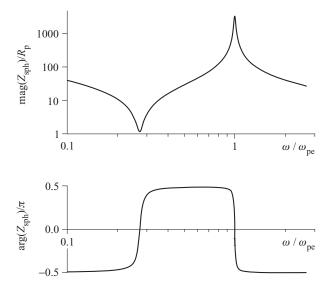
Figure 10.21 Magnitude and phase of the impedance of a floating spherical probe in a large spherical plasma-filled cavity, calculated for a uniform plasma  $(n = 10^{16} \text{ m}^{-3} \text{ and } kT_{\text{e}} = 2 \text{ eV})$ . The lower resonant frequency depends on the dimensions of the probe and its sheath:  $\omega = (s/r_0)^{1/2} \omega_{\text{pe}}$ .
