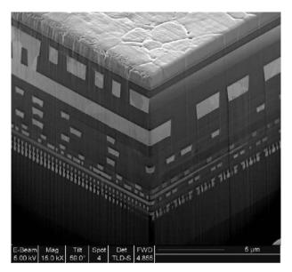
Figure 1.1 Multilevel metal dielectric interconnects in VLSI circuits.
