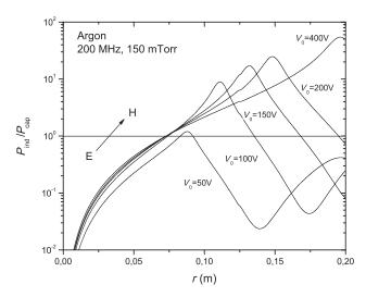
Figure 6.22 Inductive-to-capacitive power ratio,  $P_{ind}/P_{cap}$ , vs. radius for the same conditions as in Figure 6.21. The spatial E–H transitions are clearly seen at high voltage. From [21].
