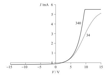
Figure 10.5 Current–voltage (I-V) characteristics (Eq. (10.2)) obtained with two asymmetrical planar probe arrangements (area ratios 34 and 340) in a low-pressure hydrogen plasma – see Exercise 10.3.
