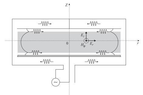
Figure 6.6 Schematic of wave propagation in a capacitive discharge operated in the electromagnetic regime.
