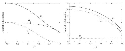
Figure 9.6 Charged particle density profiles for  $\alpha_0 = 1$  (left) and  $\alpha_0 = 10$  (right). The pressure was chosen such that  $l/\lambda_i = 10$ . The electron temperature is 3.1 eV for  $\alpha_0 = 1$  and 3.6 eV for  $\alpha_0 = 10$ .
