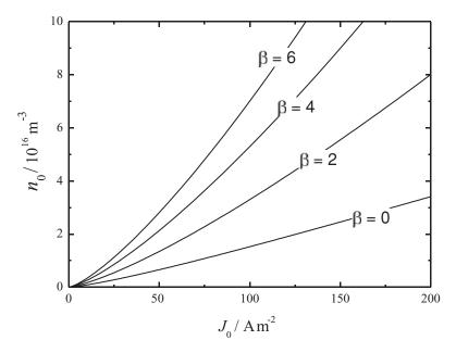
Figure 6.2 Electron density as a function of the low-frequency current density amplitude  $J_0 = I_0/A$ , for different values of the ratio  $\beta$ . The argon gas pressure was 1.33 Pa, the electrode spacing was 5 cm, the low frequency was 13.56 MHz and the high frequency was 149.16 MHz, i.e.,  $\alpha = 11$ .
