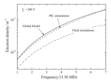
Figure 5.12 Electron density as a function of the driving frequency, as calculated by a PIC simulation, a fluid simulation and the global model. The RF voltage amplitude is fixed at  $V_0 = 200$  V, the argon gas pressure is 19.5 Pa and the electrode gap is 3 cm. From [75].
