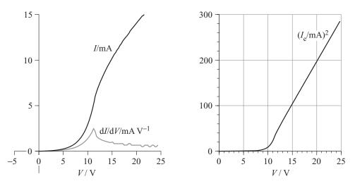
Figure 10.9 Left: The electron current to a cylindrical probe of area  $2.0 \times 10^{-5}$  m<sup>2</sup> in the same plasma as that for Figure 10.3 and its derivative, plotted against probe voltage. Right: The same probe current plotted as the square of the electron component of the current against voltage.
