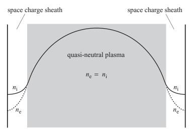
Figure 3.2 Schematic representation of a bounded plasma. The quasi-neutral plasma is separated from the walls by space charge sheaths. It is convenient to show the electrodes in a vertical orientation – in practice, gravity is unimportant and the orientation has no impact on the structure of the plasma, or of the sheaths.
