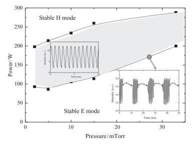
Figure 9.9 Instability window in the power/pressure space for a  $CF_4$  inductive discharge. Originally from [124].
