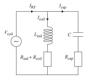
Figure 7.12 Simplified lumped element circuit model of an inductive discharge with capacitive coupling. From [125].  $R_{cap}$  accounts for capacitive heating of electrons (both ohmic and stochastic).
