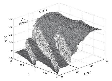
Figure 9.14 Periodic formation and propagation of double layers in the expanding chamber of an inductive/helicon plasma source working with Ar/SF<sub>6</sub> mixtures.
