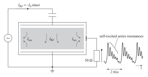
Figure 10.22 The self-excited resonance probe is effectively an isolated section of wall that takes a sample of the current flowing in the walls of the vessel, converting it to a voltage signal for analysis.
