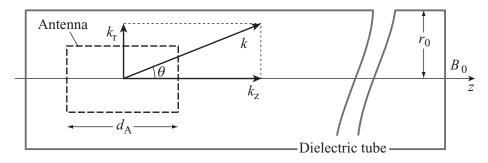
Figure 8.6 Schematic of the helicon antenna around the source tube, with wavenumbers.
