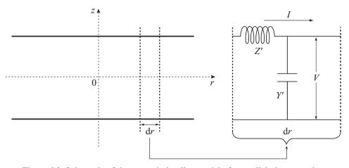
Figure 6.9 Schematic of the transmission line model of a parallel plate capacitor for VHF, showing the inductance and capacitance contributed by a radial element between r and r + dr.
