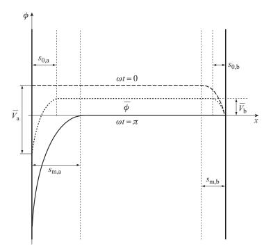
Figure 5.15 Potential V(x, t) between the electrodes for two different times during the RF cycle, along with the time-averaged value, in the case of an asymmetric capacitive discharge.  $\overline{V}_{b} - \overline{V}_{a}$  is the self-bias voltage.
