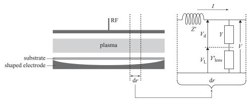
Figure 6.15 The lens concept employs a shaped electrode behind the substrate to suppress the standing wave effect (left) and the equivalent transmission line model (right).
