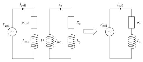
Figure 7.9 The transformer model of an inductive discharge. On the right, the secondary circuit has been transformed into its series equivalent in terms of the primary circuit current.
