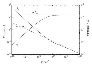
Figure 7.8 Plasma resistance and plasma current as a function of the electron density for  $v_{\rm m}/\omega = 0.1$ . We have chosen N = 5,  $I_{\rm coil} = 3$  A,  $r_0 = 0.065$  m and l = 0.3 m.
