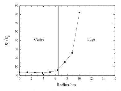
Figure 9.7 Negative ion fraction as a function of the radius in a magnetized helicon plasma in  $SF_6$ . The solid line at 6.5 cm separates the central region (where the helicon wave energy is absorbed) from the diffusion region near the edge. From [190].
