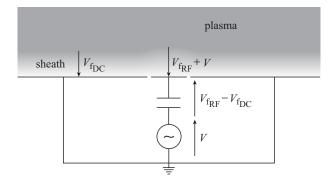
Figure 4.10 Distribution of DC and RF potentials assuming that the area of the RF-driven electrode is small compared with the ground area and that external capacitance is sufficiently large for it to have negligible RF impedance compared with the electrode sheath;  $V = V_1 \sin \omega t$ .
