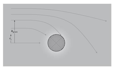
Figure 10.8 Trajectories of particles with the same energy, starting with different impact parameters. Those with  $h \le h_{\text{graze}}$  are collected by the probe; those with  $h > h_{\text{graze}}$  miss the probe.
