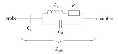
Figure 10.20 The equivalent circuit of the spherical probe in Figure 10.19.
