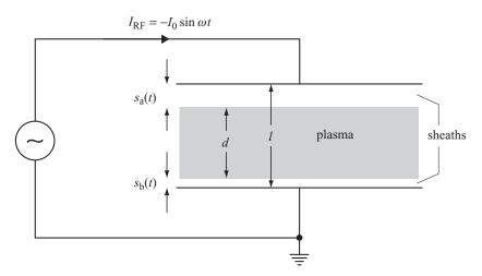
Figure 5.1 Schematic of the symmetrical capacitive discharge model. The definition of the current is chosen to simplify the analysis.
