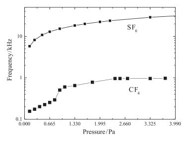
Figure 9.10 Frequency of the oscillations measured in CF<sub>4</sub> and SF<sub>6</sub>.
