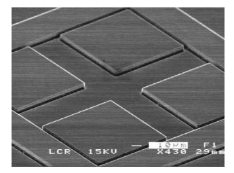
Figure 1.4 Deep micrometre-scale structure etched in SiC using a  $SF_6/O_2$  helicon plasma.
