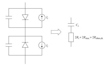
Figure 5.5 The electric circuit model for the two sheaths considered separately (left) and combined (right).
