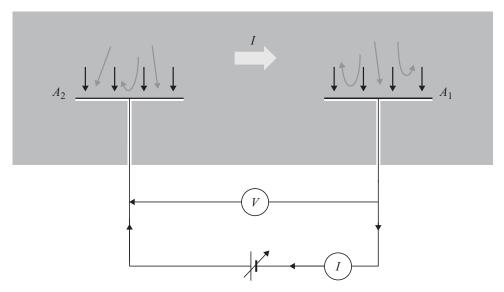
Figure 10.2 Two surfaces linked by a battery – the potential is distributed in order that the current is continuous. It is supposed that the lower surfaces are insulated from the plasma, so current is collected only on the upper surfaces. I(V) is given by Eq. (10.2).
