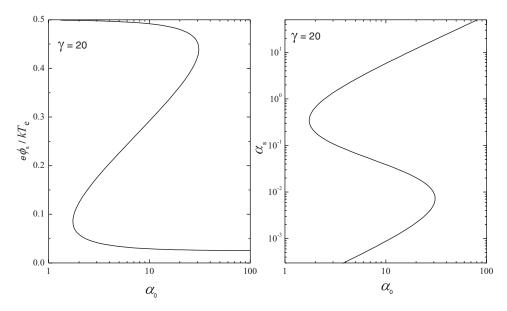
Figure 9.4 Negative ion fraction at the sheath edge,  $\alpha_s$ , and potential drop in the presheath,  $\phi_s$ , as a function of the negative ion fraction at the centre,  $\alpha_0$ .
