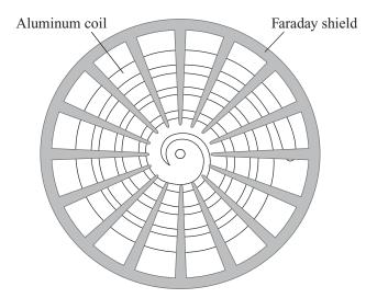
Figure 7.19 View of a Faraday shield for a planar coil, seen from the side of the dielectric window. From [130].
