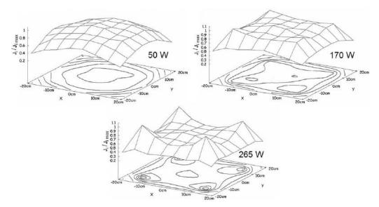
Figure 6.23 Ion flux mapping over the electrode for a 60 MHz discharge driven at different powers. Inductive heating is observed near the edges. From [91].
