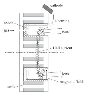
Figure 1.6 Schematic of a Hall effect thruster.
