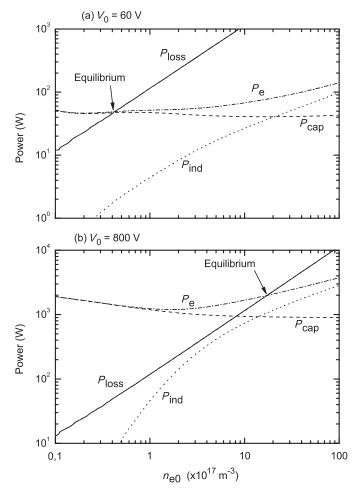
Figure 6.18 Contributions to power absorption and the power loss term as a function of central electron density,  $n_{e0}$ , for a 4 Pa (30 mtorr), 200 MHz capacitive discharge with electrodes of radius  $r_0 = 15$  cm separated by l = 4 cm, for (a)  $V_0 = 60$  V and (b)  $V_0 = 800$  V. From [21].
