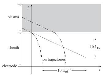
Figure 4.2 Schematic ion trajectories (dashed lines) in a steady sheath: ions approach the sheath boundary close to the Bohm speed, being significantly accelerated when inside the sheath.
