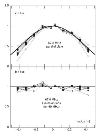
Figure 6.16 Experimental evidence of the suppression of the standing wave effect using the shaped electrode and lens concept. From [110].
