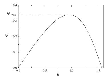
Figure 8.5 The angle between the ray direction (group velocity vector direction) and the magnetic field direction,  $\psi$ , as a function of  $\theta$ . A maximum angle  $\psi_{\text{res}} \approx 0.33$  is reached when  $\theta \approx 0.95$ . The angular limitation of the ray direction accounts for the tendency of helicon waves to follow the magnetic field lines.
