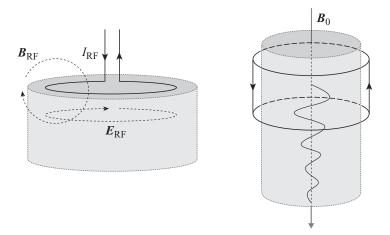
Figure 1.8 Cylindrical columns of plasma excited by external currents. Left: the plasma is sustained with currents driven by the RF electric field induced in the plasma in response to external RF current – the field strength diminishes with distance from the external coil. Right: the external antenna sets the current path such that helicon waves are launched, propagating axially – the plasma is sustained by energy absorbed from these waves.
