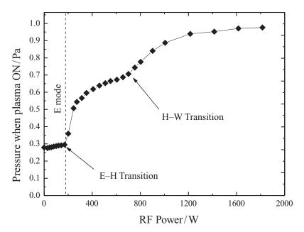
Figure 8.9 Gas pressure measured at the wall of a  $SF_6$  plasma produced in a helicon reactor. The E–H and H–W transitions are identified as the power increases.
