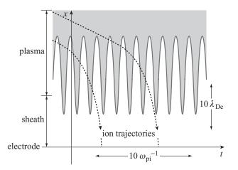
Figure 4.4 Schematic ion trajectories in a temporally modulated sheath  $(\omega \sim 5 \omega_{pi})$ : ions approach the sheath boundary close to the Bohm speed, being significantly accelerated when inside the sheath and being repeatedly overtaken by the oscillating sheath.
