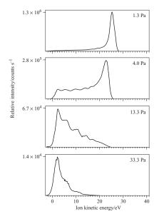
Figure 4.7 Argon ion energy distributions at the grounded electrode of a 13.56 MHz plasma with low power input ( $\sim 2$  W) in a CCP between 10 cm diameter plates, 2.5 cm apart [49].
