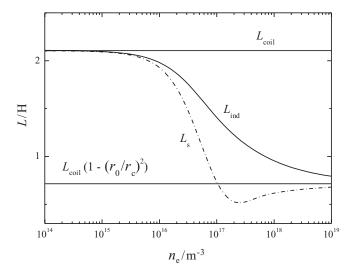
Figure 7.10 Inductance of the transformer model,  $L_s$ , along with the inductance derived from the electromagnetic model,  $L_{ind}$ , as a function of the electron density for  $v_m/\omega = 1$ . We have chosen N = 5,  $r_0 = 0.065$  m,  $r_c = 0.08$  m and l = 0.3 m.
