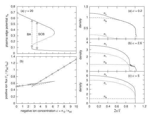
Figure 9.5 On the left, the potential drop in the presheath and normalized flux at the wall as a function of  $\alpha_0$ . On the right, the density profiles in the three regimes. From results of numerical simulations in [175].
