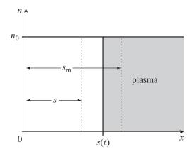
Figure 4.12 An RF ion matrix sheath; the ion density is constant throughout at  $n_0$  and s(t) is the instantaneous sheath width, so that  $n_e = n_0$  for x > s(t);  $s_m$  is the maximum sheath extent and  $\overline{s}$  is the mean sheath width.
