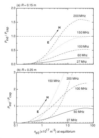
Figure 6.19 Inductive-to-capacitive power ratio,  $P_{ind}/P_{cap}$ , vs.  $n_{e0}$  at equilibrium, for several frequencies and for (a)  $r_0 = 15$  cm and (b)  $r_0 = 25$  cm. The other conditions are similar to that in Figure 6.18. From [21], where the frequency unit should be MHz and *R* is equivalent to  $r_0$  in this text.
