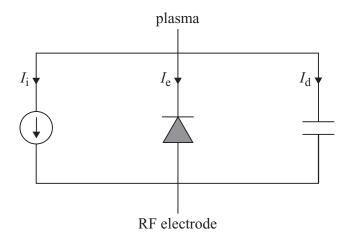
Figure 4.11 A schematic circuit model of an RF sheath featuring a constant current source (ion current), a reverse-biased diode (electron current) and a non-linear capacitor (displacement current). The ion source and diode will each dissipate power in proportion to the current through it and the component of in-phase voltage across it.
