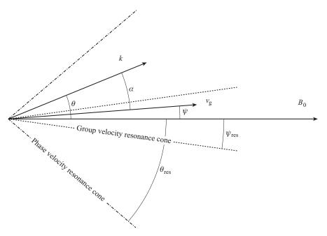
Figure 8.4 Schematic representation of the wave and group velocity vectors, limited in their respective resonance cones, of angle  $\theta_{res}$  for the phase velocity and  $\psi_{res}$  for the group velocity.
