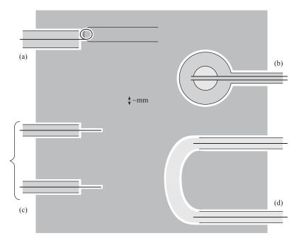
Figure 10.18 Various types of microwave probes in cross-section: (a) hairpin resonator (the hairpin is supported in a plane slightly behind that of the loop, from which it is DC-isolated); (b) multipole resonator; (c) transmission cut-off; (d) surface waveguide.
