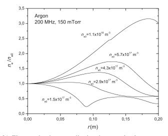
Figure 6.21 Electron density normalized to its central value  $n_{e0}$  vs. radius for various RF voltages (and thus various  $n_{e0}$ ). The frequency is 200 MHz, the argon pressure is 20 Pa and the electrode radius is  $r_0 = 0.15$  m. From [21].
