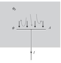
Figure 10.1 Particle fluxes to a surface (area A, potential  $\phi$ ) immersed in plasma (potential  $\phi_p > \phi$ ) – electron flux is indicated in grey, ion flux in black. Imbalance between the fluxes forms a net current *I*. It is supposed that the lower surface is insulated from the plasma, so current is collected only on the upper surface.
