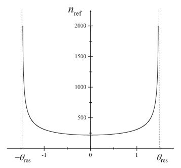
Figure 8.3 Refractive index as a function of  $\theta$  in radians; the propagation is restricted within the phase velocity resonance cone of angle  $\theta_{\rm res}$ . The following conditions were used: f = 13.56 MHz,  $B_0 = 0.005$  tesla and  $n_e = 10^{18}$  m<sup>-3</sup>.
