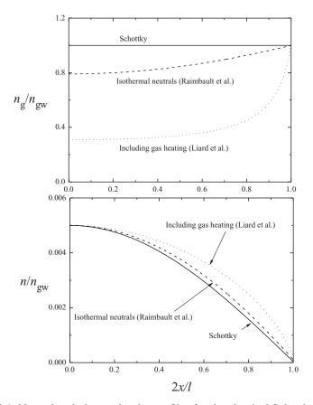
Figure 9.1 Neutral and plasma density profiles for the classical Schottky model, the neutral depletion model of Raimbault *et al.* and the model of Liard *et al.* that includes gas heating.
