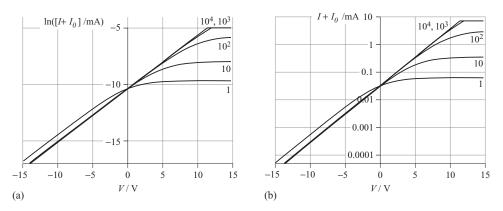
Figure 10.6 (a) The semi-log plot of electron current (in mA) at the probe electrode for reference electrodes having area ratios 1, 10,  $10^2$ ,  $10^3$  and  $10^4$ , in the same plasma as that for Figure 10.3; (b) the same data presented as a plot of current on a  $\log_{10}$  scale.
