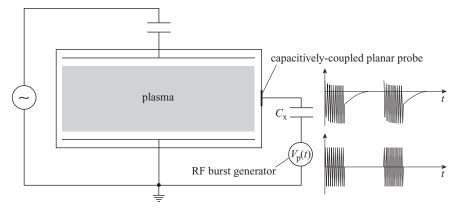
Figure 10.13 Schematic diagram of a self-biased planar probe, embedded in a grounded surface. The probe bias is derived from a burst of RF applied to the probe, during which a self-bias voltage is established across the external capacitance  $C_x$ . At the end of the burst the RF is switched to zero and the capacitor discharges at a rate initially determined by the flux of positive ions from the plasma onto the probe.
